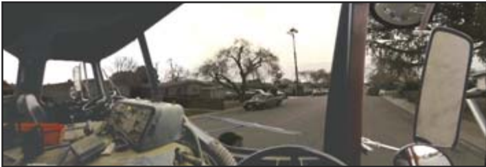
Digital computer model of garbage truck interior used in visibility study
