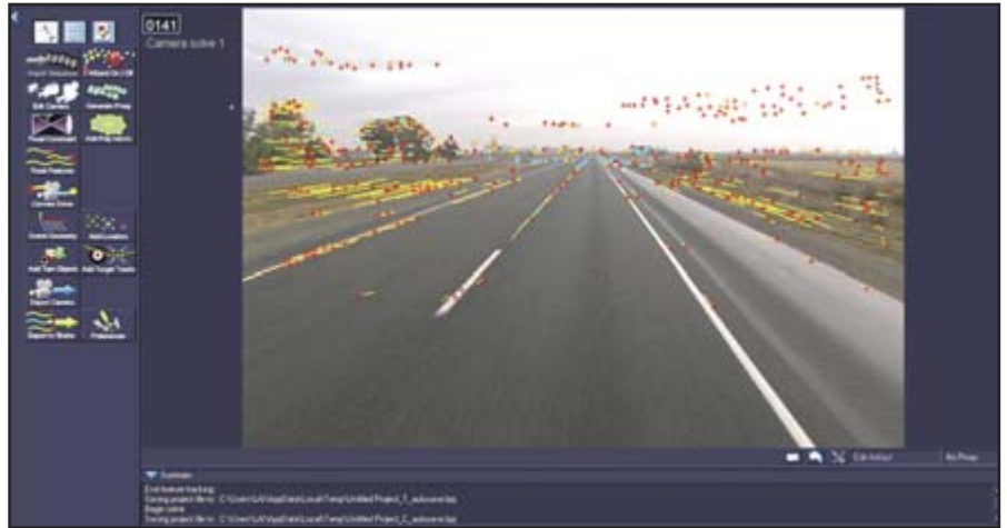
3D camera matching software tracking 2D features
